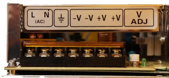
1. Wire the V- to the Power – terminal on the SlushEngine ( Located in the bottom right of the board )
