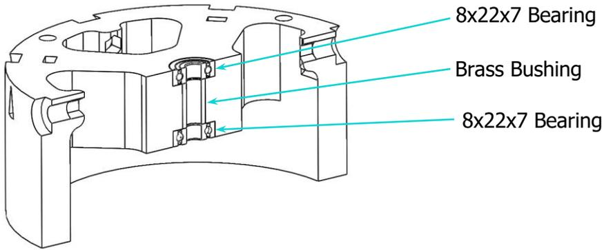
1. Insert the large brass bushing into the base
