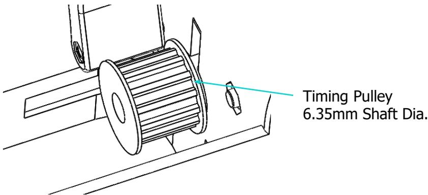
1. Place the pulley onto the shaft of the motor
