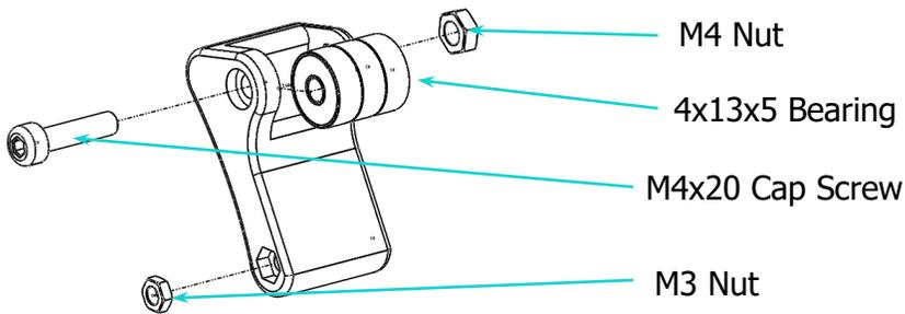
1. Place 3 bearings into the pocket on the tensioner print
