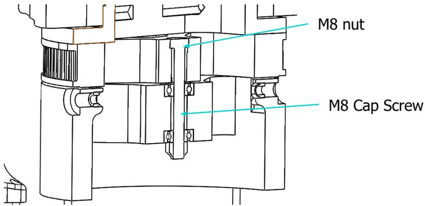
1. Assemble the shoulder gear to the base by running the M8 bolt through the brass bushing and tightening the lock nut.
