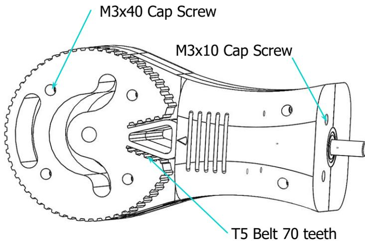
1. Place the second half of the forearm body over the stepper motor and components installed in the previous half
