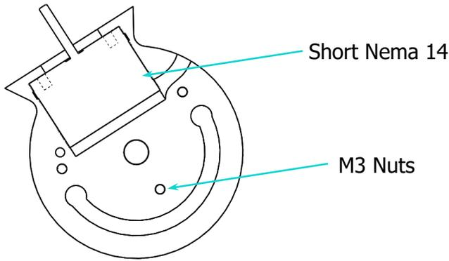
1. Insert 3 M3 Nuts into the nut traps on the other side of the wrist gear part
