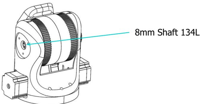
1. Drop the belts into the Shoulder body and loop the belts around the timing pulleys
