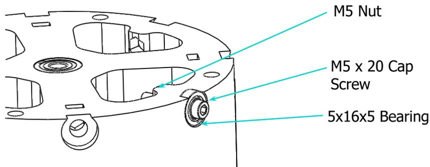
1. Insert M5 nuts into all nut traps on the inside of the base
