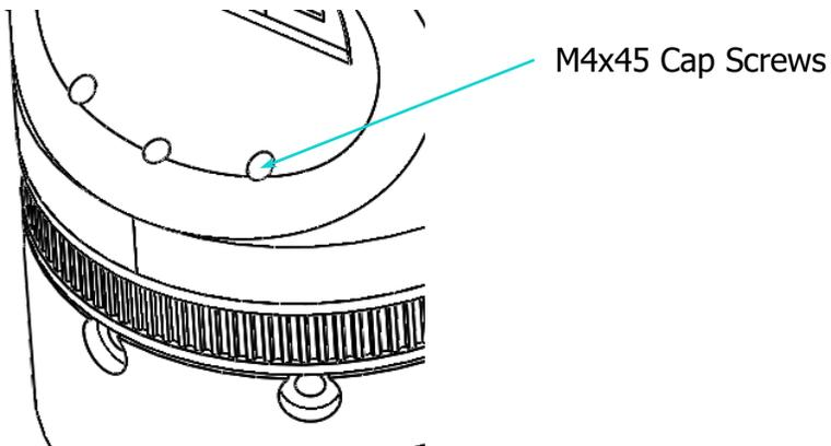
1. Drop M4x45 cap screws down into the holes and then align with nuts on shoulder gear below. Tighten these to assemble the shoulder to the base
