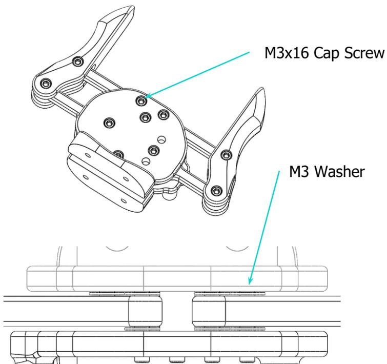
1. Fasten all M3x16 cap screw into each of the available holes
