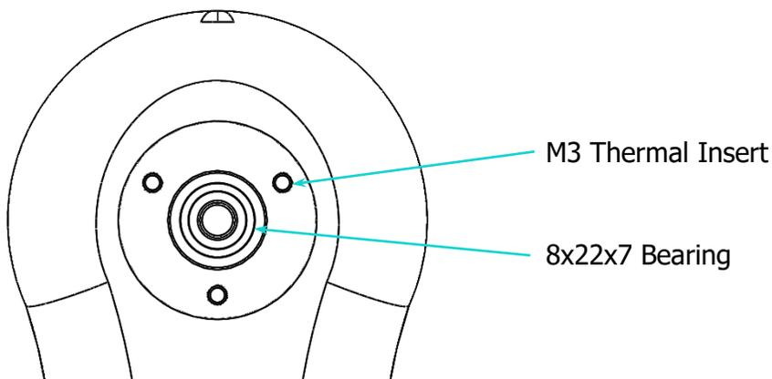
1. Install the M3 Thermal inserts on both sides. 6 should be installed in total
