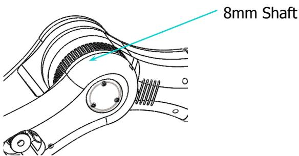
1. To assembled the forearm to the arm use the same technique that was used when assembling the shoulder gears
