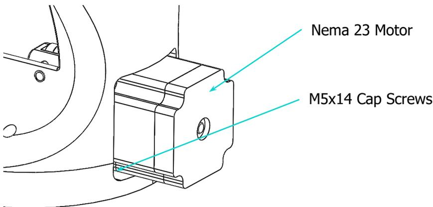
1. Insert the motor into the side of the shoulder body
