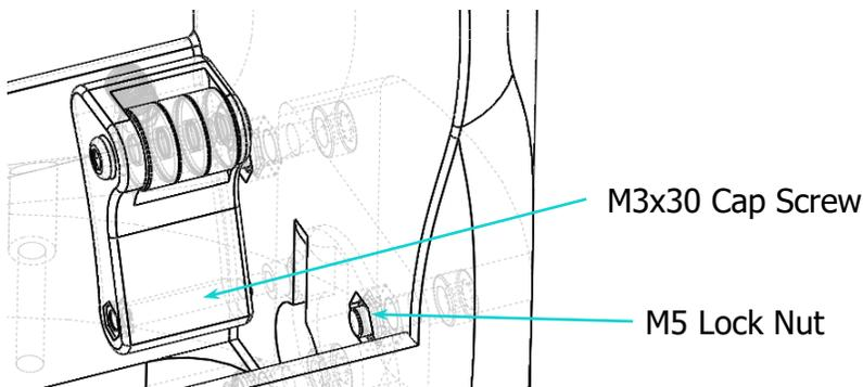
1. Place 4 M5 Lock nuts in the nut traps for the motor mounting. Do this on each side of the shoulder
