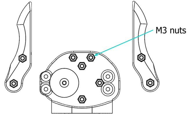
1. Insert 11 M3 Nuts into their respective nut traps
