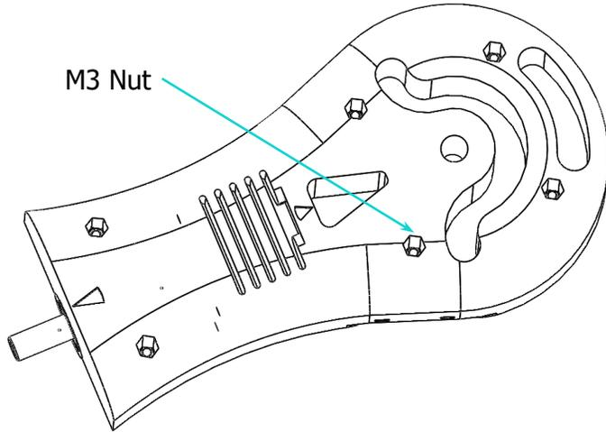
1. Insert 6 M3 nuts into the nut traps on the half of the Forearm body
