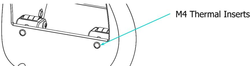
1. Place the thermal insert on the end of a soldering iron
