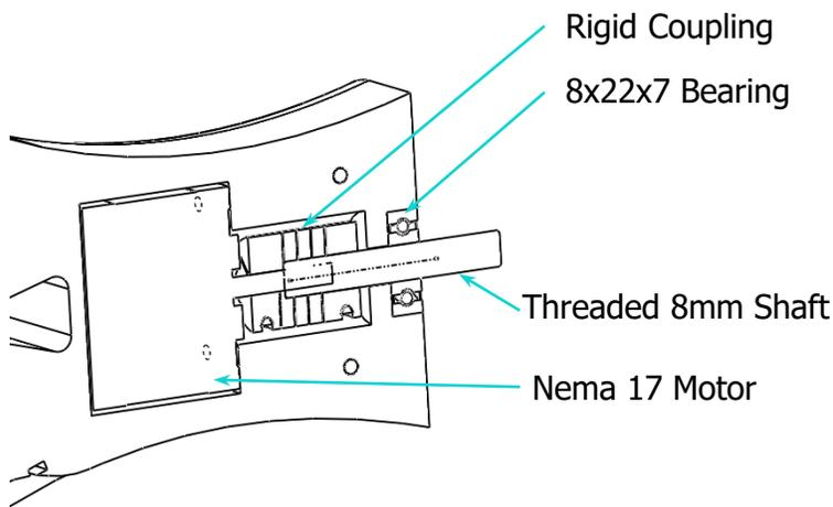
1. Attach the stepper motor to the rigid coupling
