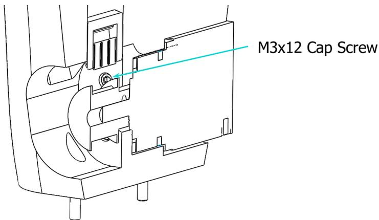
1. Install the geared motor using M3 cap screws
