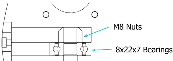
1. Slide the bearing into the trap hole. Look at the bottom of the wrist body to make sure the bearing hole is aligned correctly
