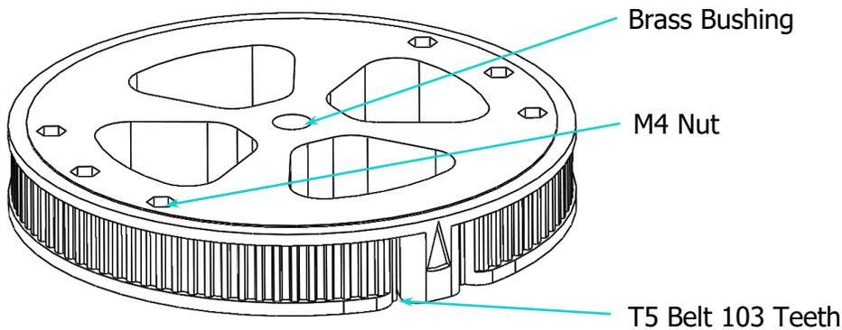
1. Press in the second brass bushing into the base gear
