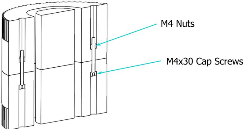
1. Drop 4 M4 Nuts into the nut traps on the Shoulder gear
